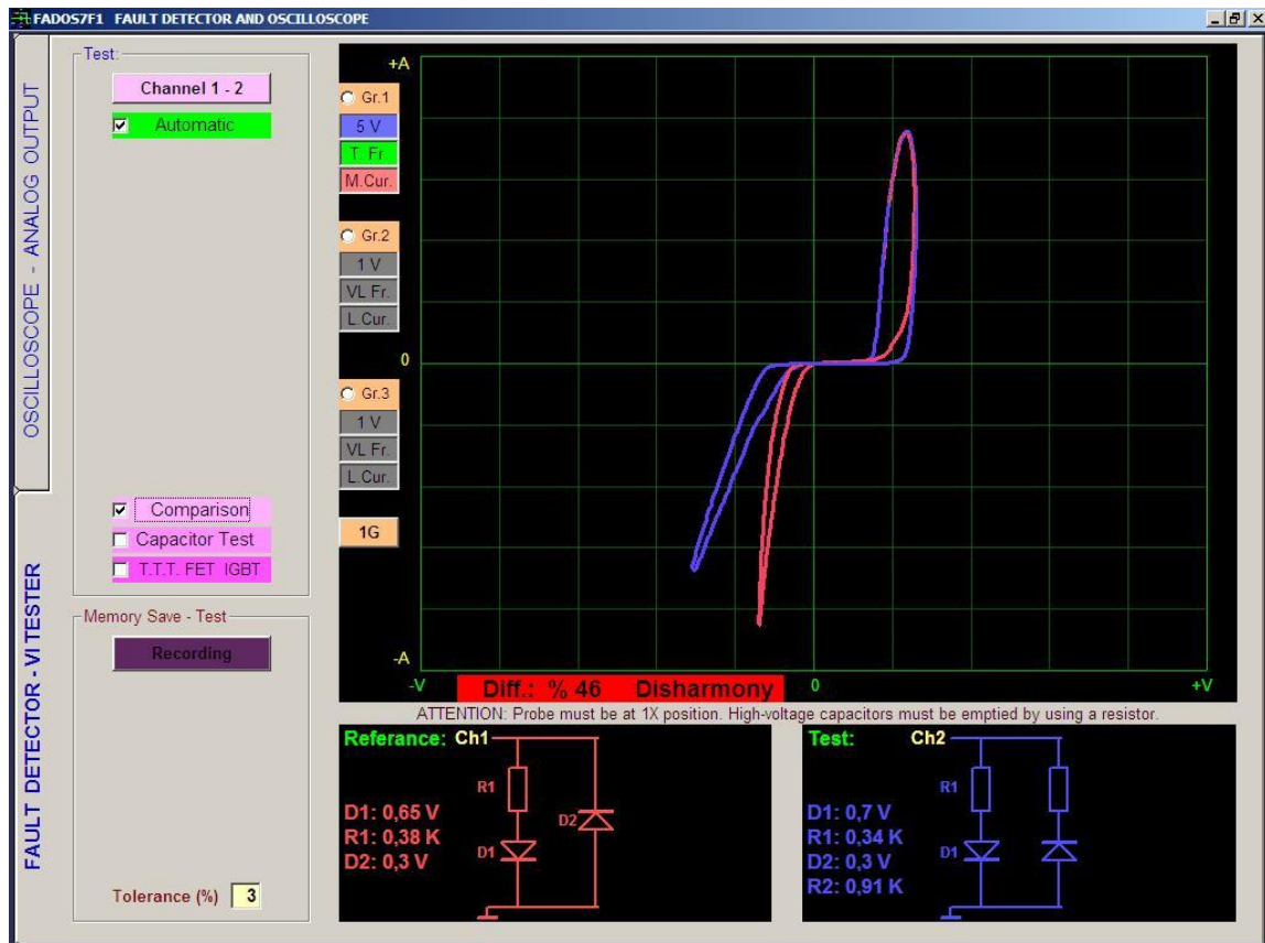
Picture 25: Comparison Test – Integrated Pin Faults
