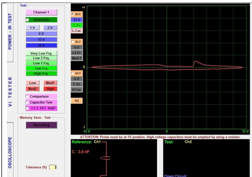
Figure 147: Gate (+) Emitter (-) VI Graph
