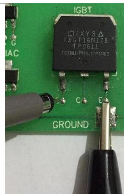
Figure 148: Channel1 Probe Used for Gate - Emitter Measurement
