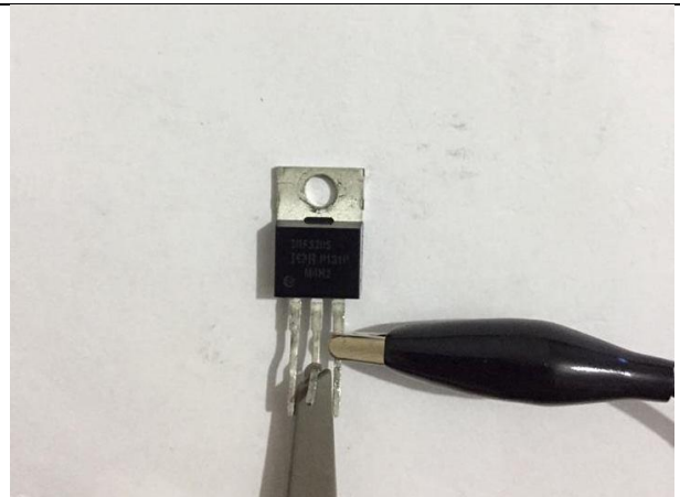
Figure 136: Channel1 Probe Used for Drain - Source Measurement
